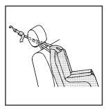
If the position you are using has an adjustable head restraint and you are using a dual tether, route the tether under the head restraint and in between the head restraint posts.
